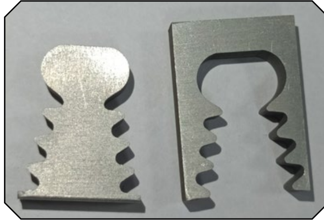
Aerospace Parts Manufacture using Wire-EDM Process
