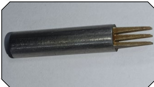
Multi-micro-tip electrode Fabricated using Wire-EDM Process
